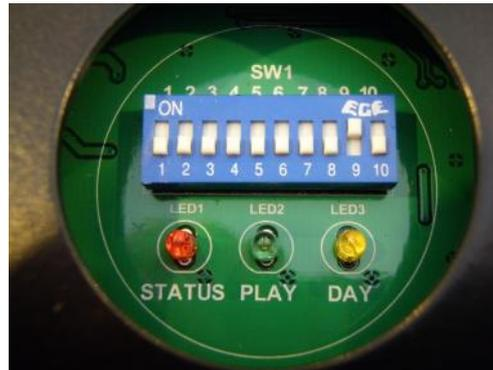
The six mini switches numbered 1 to 6 are used to select the bird distress calls to be broadcast. The normal allocation of bird species to each switch is as follows:
