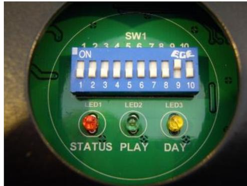
The Test Mode switch is number **10** on the mode switch block. This switch should only be set to ON when making control panel adjustments and must be left in the downward OFF position after installation is complete. When set to ON, the following times apply:
