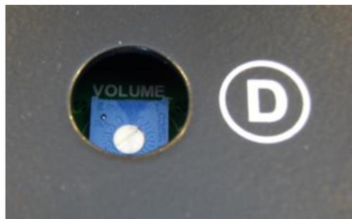
2. Use the *Control Adjustment Tool* to turn the small white screw in the centre of the blue volume switch (see above) from fully anticlockwise (which is zero volume) by roughly 10° intervals. The maximum volume is achieved when the screw is turned fully clockwise.
