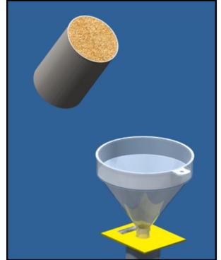
4. Hold the funnel spout level with the top of the cylinder, slide away the plastic insert and allow the cylinder to fill with grain.
