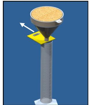
5. Using the plastic card, slide off any excess grain to leave a level top. Do not tap the cylinder or consolidate the grain in any way.
