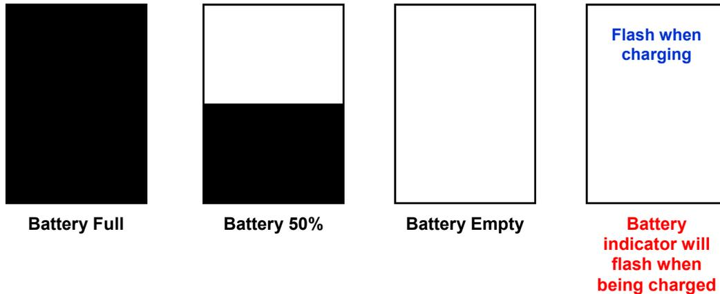
If the battery should go flat while weighing a **LOW BATTERY** warning will flash in the display and the weigher will eventually turn off. Data already stored in the weigher will remain in memory even if the unit automatically turns off.
