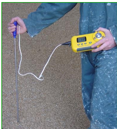
Grain temperature measurement with the Protimeter 1.5m temperature probe
