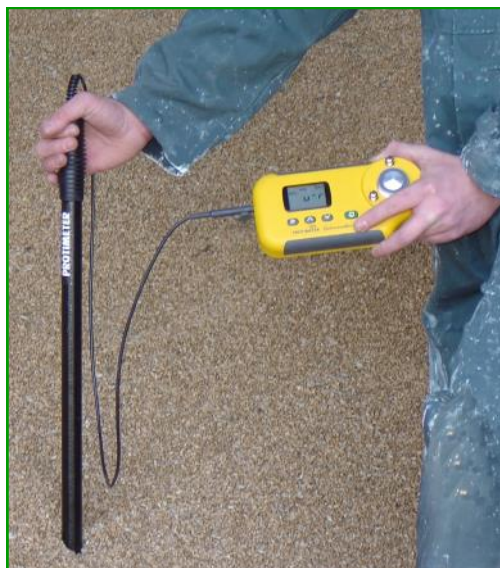
In-heap measurement with the Protimeter
